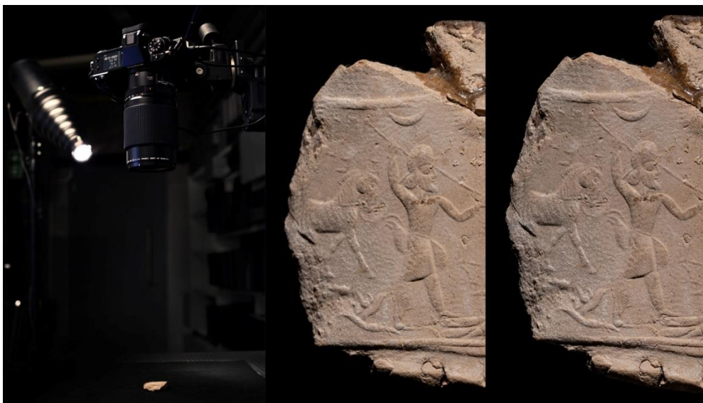
Combining focus-stacking and photometric stereo. Though the thickness of the seal is a mere 7.5mm, limited depth-of-field due to recording at such a high magnification only allows for acceptably sharp capture of the top 2mm. The benefits of focus stacking are particularly notable at the edges of the seal as they taper down. Left: single exposure. Right: focus-stacked image. Sigill. Aram. V.
