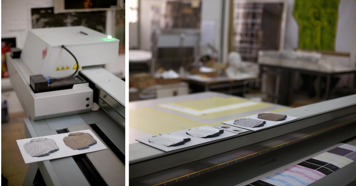
Left: Two, scaled-up, 3D printed facsimiles of Sigill. Aram. V, made in the print rooms at Factum Arte, Madrid. Right: The two tiny facsimiles in the centre of the group are printed at actual size. Variations of enlarged facsimiles were produced, either uncoloured or with renders printed on their surface.
